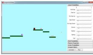
Figure 7. The technical prototype built to understand the impact of altering parameters on the player’s experience. Sliders on the right control every parameter of the generator. The area on the left allows the designer to play levels as soon as they are generated.
